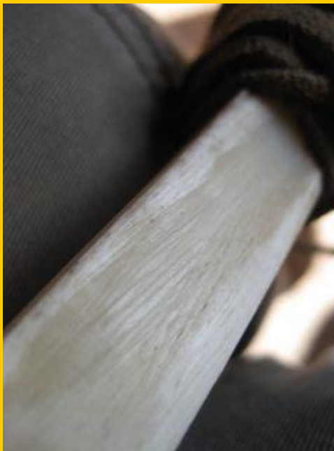
Traces of sharpening with flint blade on tool 1
